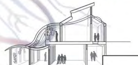
Two-Storey Classroom Section 1:100. Cluster 3 comprises a two-storey building. This helps to shield the lower 'peaceful areas' of site, from the upper noisier high-activity sports and play zones (see site section).
