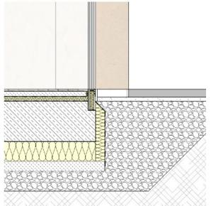
Perimeter insulation: Styrodur 2800 C foam board
