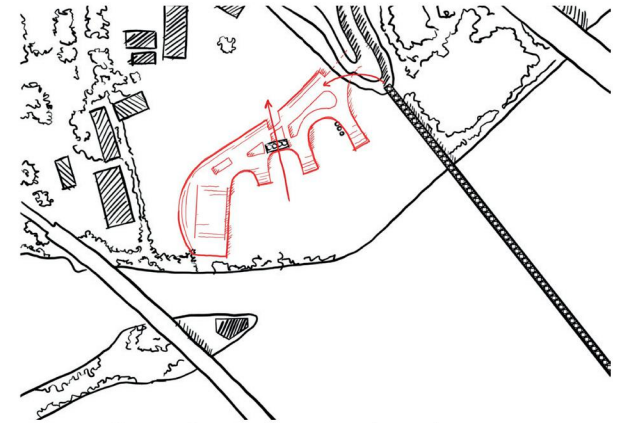
Creation of an embankment The ground rises to form a built-up area. The roof remains accessible.
