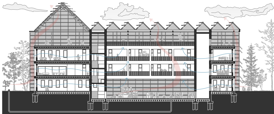
In summer, the atrium acts like a solar chimney, cooling the building.
