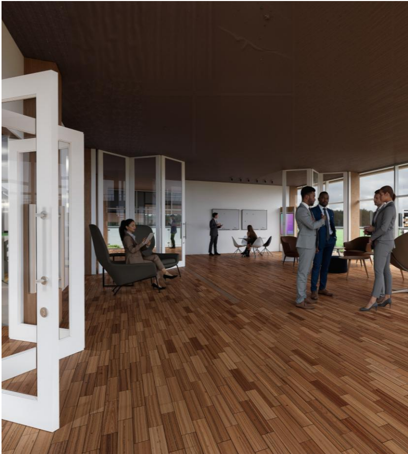
Top-hung retractable wall panels slide and stack, enabling spatial reconfiguration while maintaining acoustic separation
