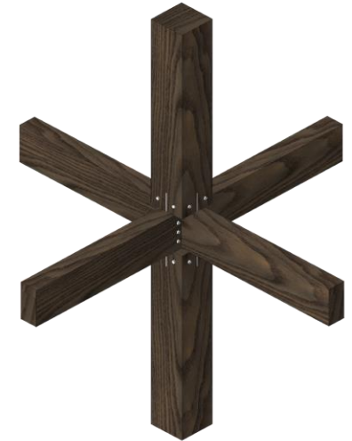
3. Then the upper column is bolted, which hides the joint within the structure when fully assembled.
