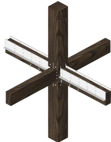
4. Steel L-shaped bracket is bolted to the beams.
