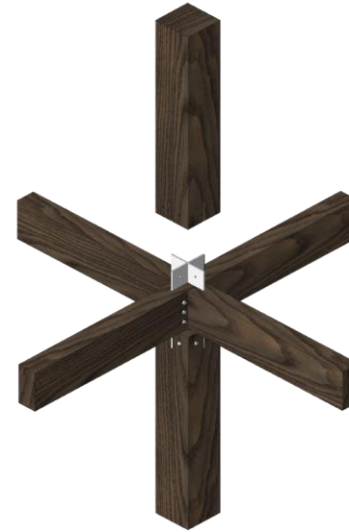
2. It is first bolted to the bottom column and then to the beams.
