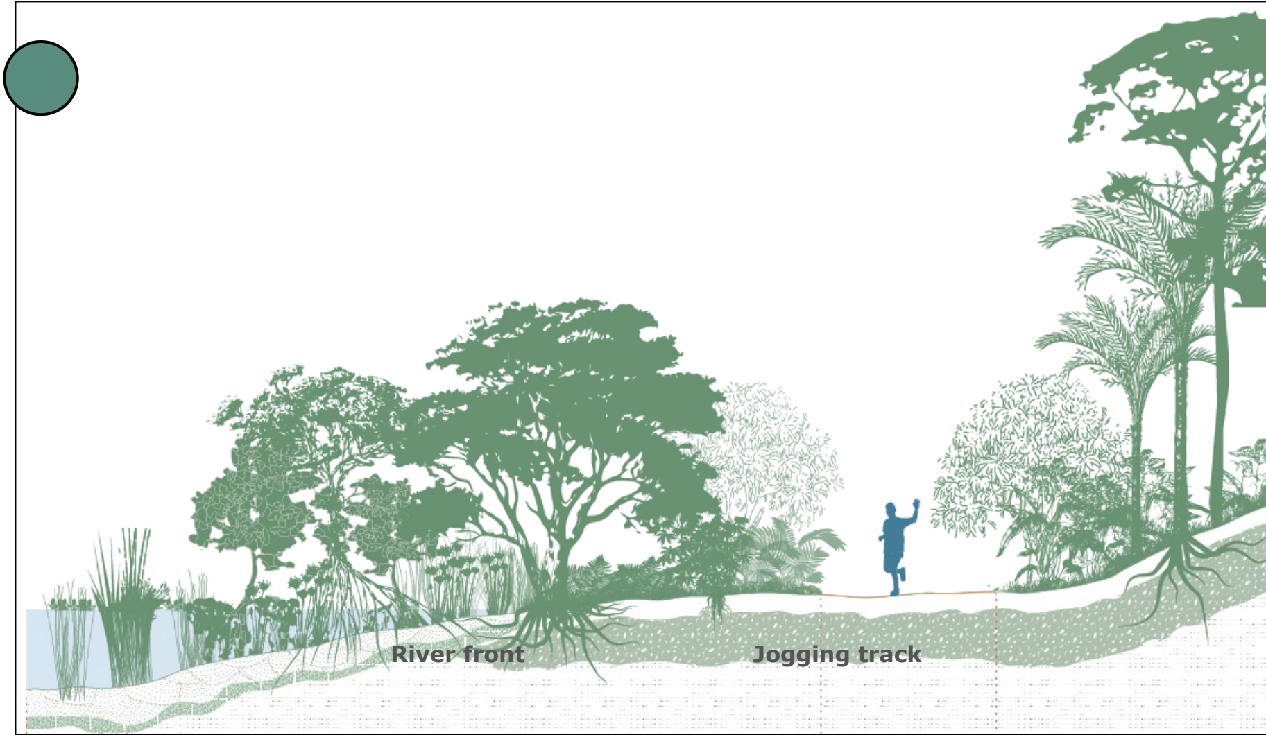
RIPARIAN BUFFER A vegetative buffer that provides a suitable distance from the river helps protecting the area near the river
