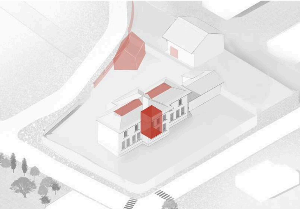
1. Placing new modular square spaces in the old building
