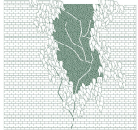
REINFORCEMENT OF WALL DEFECTS WITH VEGETATIVE MUSHROOM - MYCELIUM
